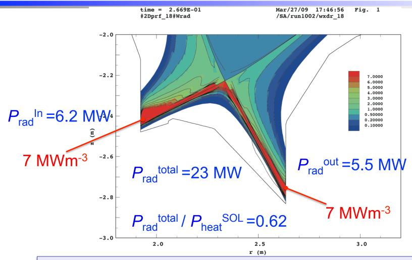
High radiation in both inner and outer divertors is predicted
