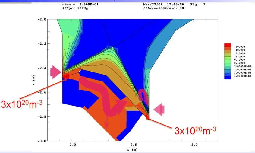
High neutral density in the V-shaped corner is predicted by SOLDOR simulation for the case with  $I_p$  of 5.5 MA,  $P_{\text{heat}}$  of 41 MW,  $\Gamma_{\text{gas}}$  of 1.5x10<sup>22</sup>/s and  $S_{\text{pump}}$  of 50 m<sup>3</sup>/s.
