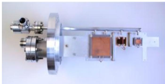
A set of electrostatic detectors
