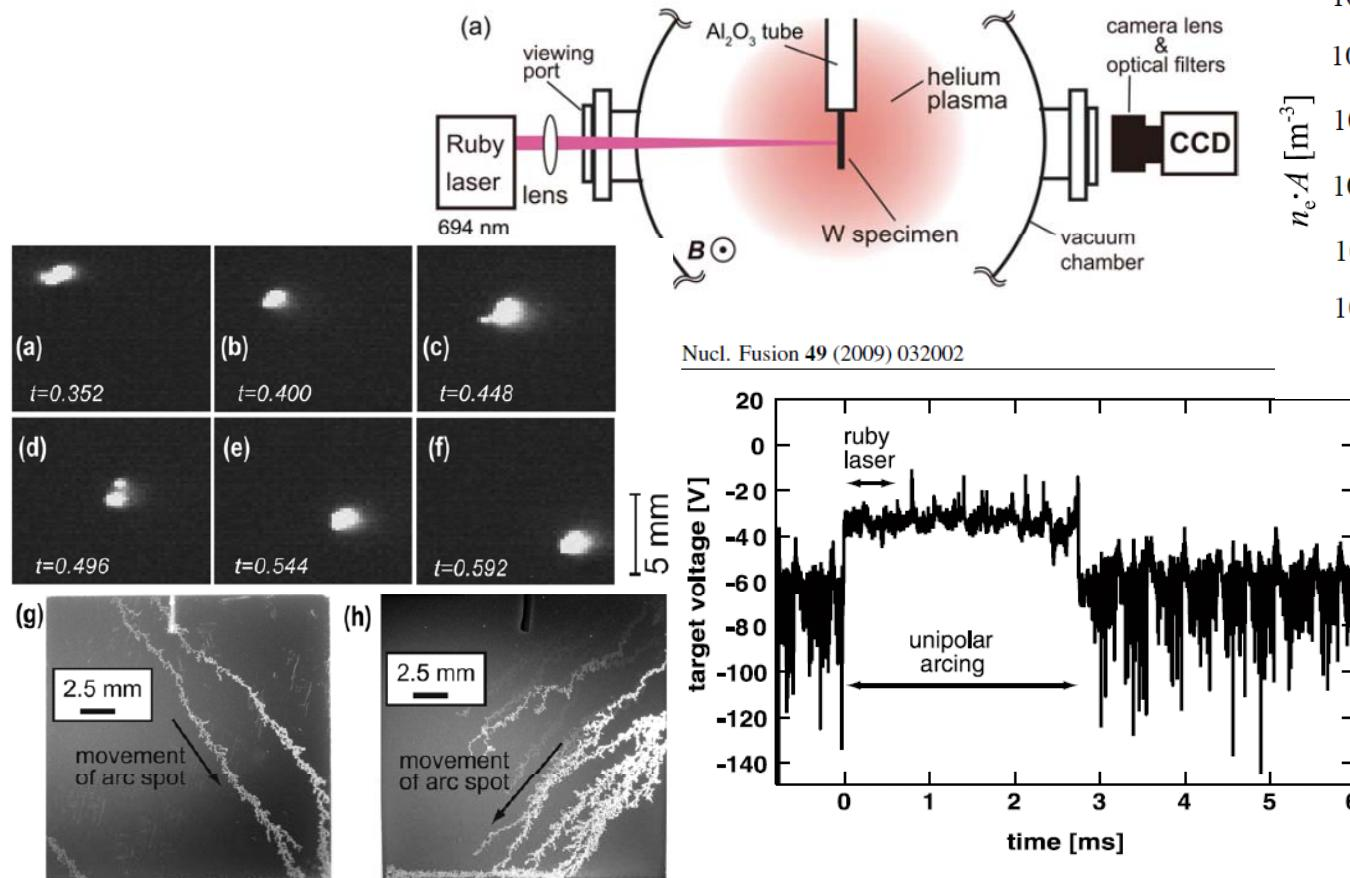
Figure 4. (a)–(f) show the temporal evolution of the emission W<sub>I</sub> ( $\lambda = 429.5$  nm) at every 48  $\mu$ s from a cathode spot running on the electrode, for the configuration for case (i). (g) and (h) are pictures of the back (the non-laser-irradiated side) of the electrode surface after the experiments with configurations (i) and (ii), respectively.
