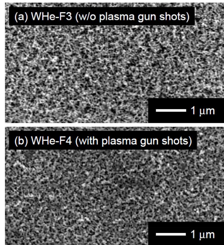
Fig. 4. SEM images of fuzzy W surfaces ( $L_{\text{fuzz}} \sim 3 \mu\text{m}$ ). (a) WHe-F3: without plasma gun shots. (b) WHe-F4: after 10 plasma gun shots with  $\sim 0.7 \text{ MJ/m}^2$  per shot.
