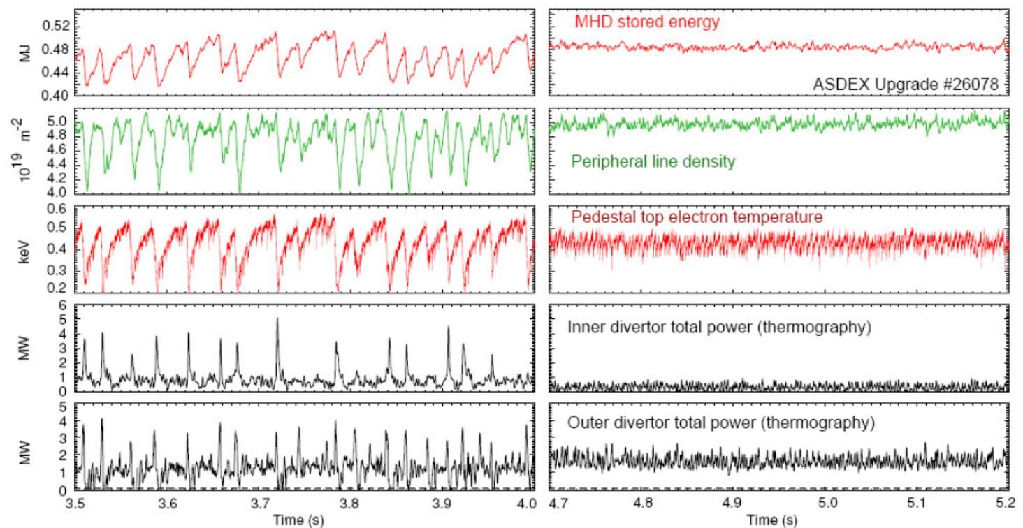
Much reduced excursions of  $W_{\text{MHD}}$ ,  $\bar{n}_e$ ,  $T_{e,\text{ped}}$ ,  $P_{\text{div}}$ !
