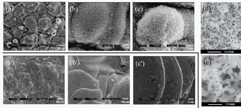
Fig. 1 (a)~(c): SEM photographs of W-C surface after and (a')~(c') before helium plasma irradiation at a surface temperature of 1250 K, a fluence of  $3.5 \times 10^{27} \text{ m}^{-2}$  and an ion incident energy of 12 eV. (d) and (e): photographs taken by FE-SEM with a high spatial resolution. The line of sight is normal to the samples.
