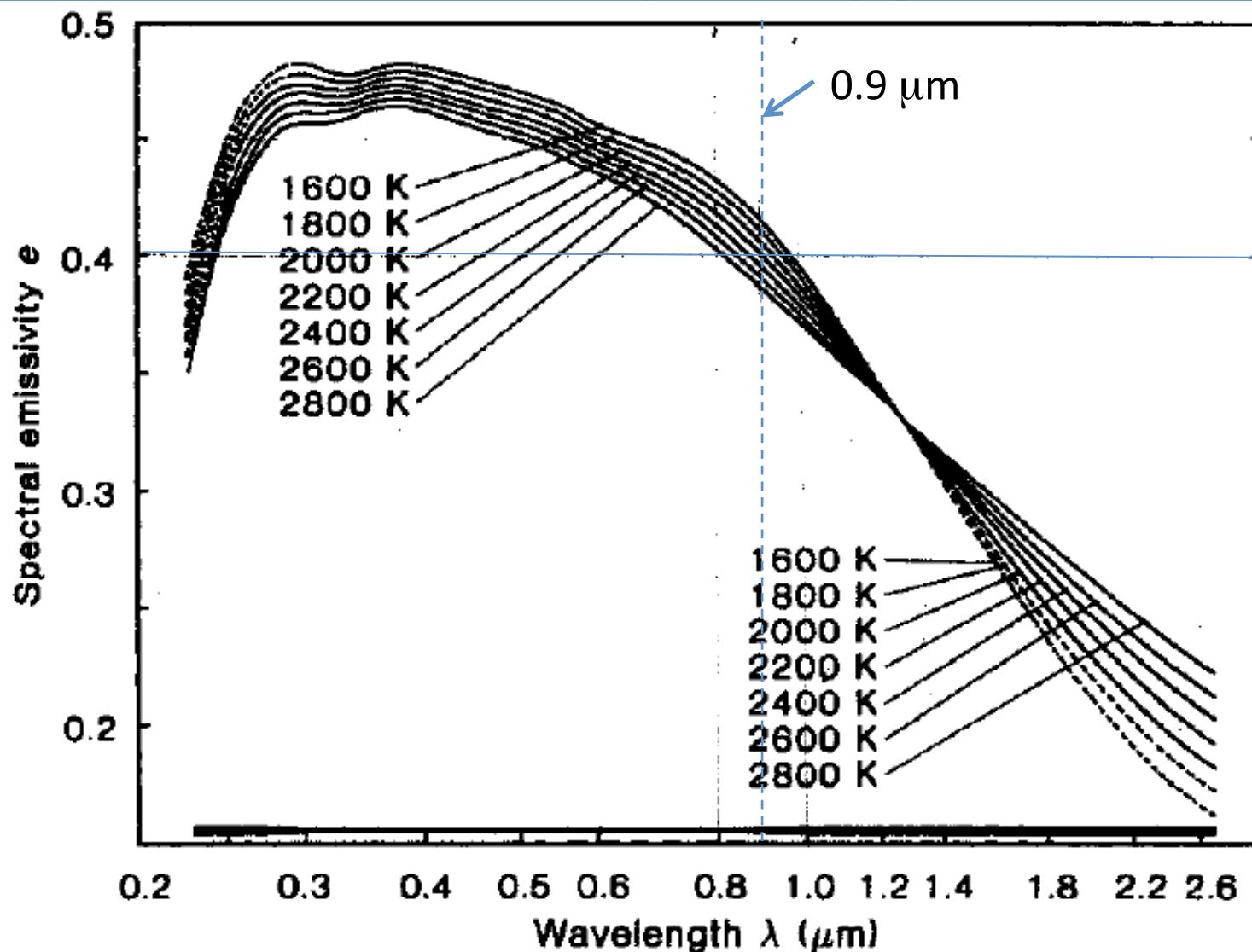
FIGURE 1.20. Spectral emissivity of tungsten according to de Vos [1.37].
