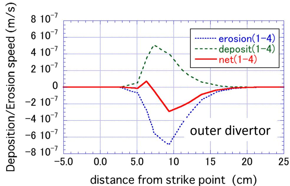
The erosion/deposition speed decreases by 2 orders of magnitude compared with the 3GW case.
