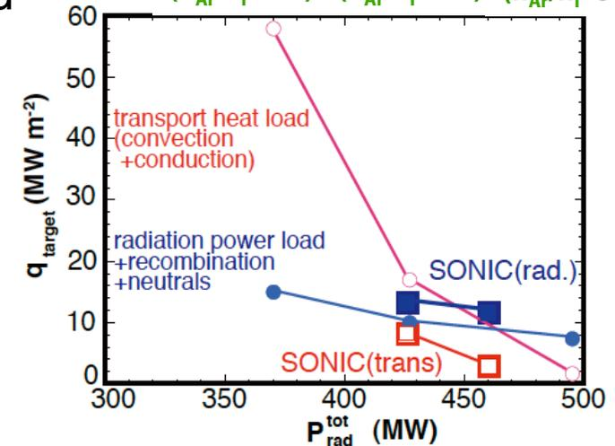
ex. Divertor geometry effect (simple impurity model)
