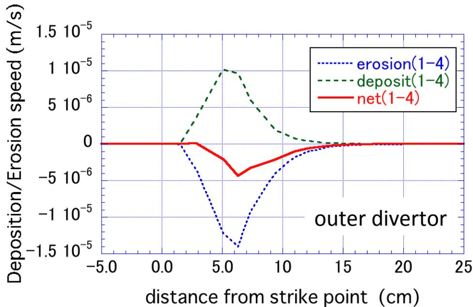
In the 1<sup>st</sup> generation, most of W particles deposit near the erosion layer.
