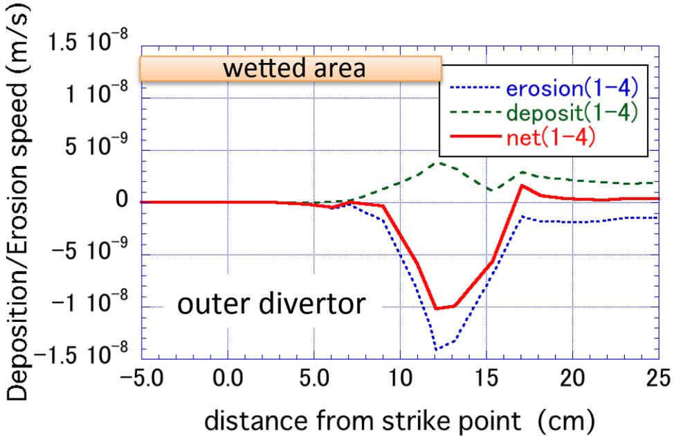
Erosion/deposition speed is much smaller than other cases.
