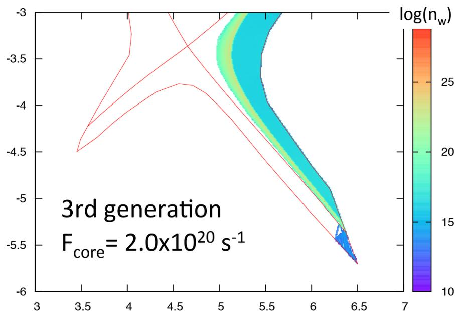
Background plasma flow and the resultant shielding effect is weak due to the high recycling. Therefore the sputtered W is easily transported upstream.
