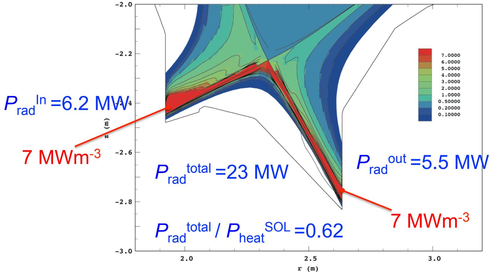
High radiation in both inner and outer divertors is predicted
