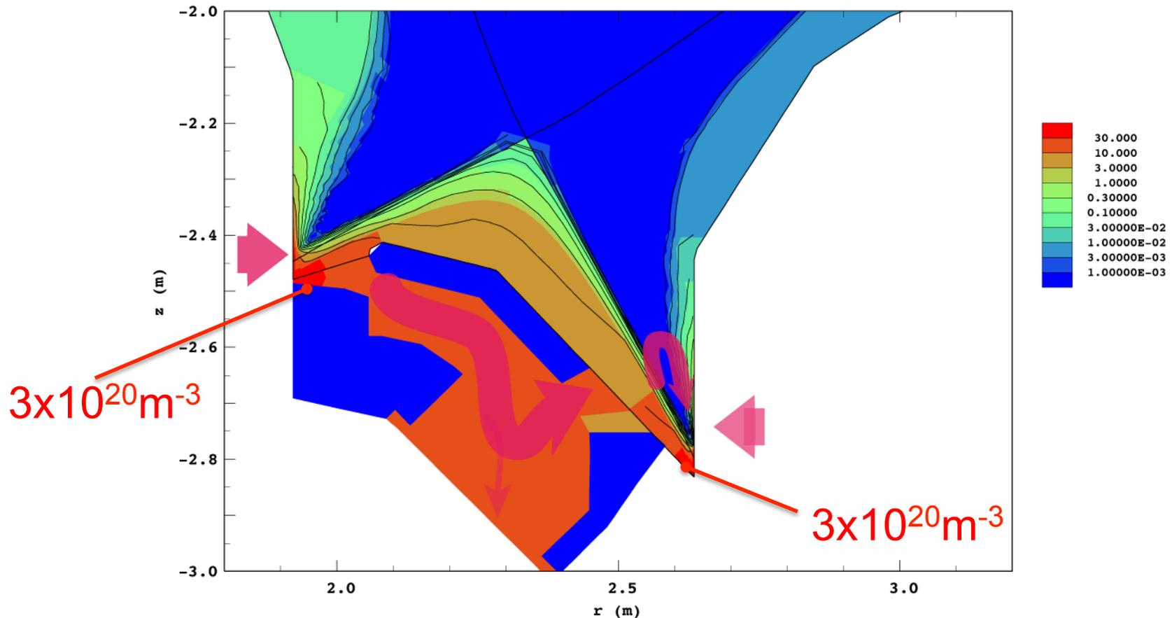
High neutral density in the V-shaped corner is predicted by SOLDOR simulation for the case with  $I_p$  of 5.5 MA,  $P_{\text{heat}}$  of 41 MW,  $\Gamma_{\text{gas}}$  of  $1.5 \times 10^{22}/\text{s}$  and  $S_{\text{pump}}$  of  $50 \text{ m}^3/\text{s}$ .
