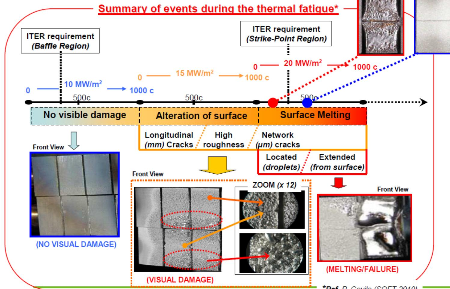
◆ Qualification of CFC/W components after Manufacturing Phase
